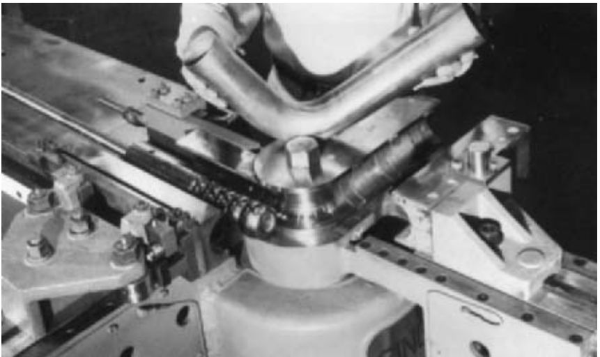
FIGURE A6.9 Tooling for a draw bend application. ( Teledyne Pines )
