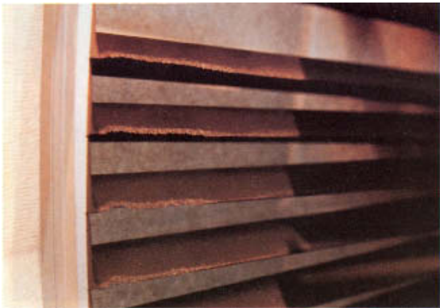
Figure 17.10 Ragged leading edges of final-stage turbine blades. Damage was caused by water-droplet impingement.
