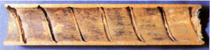
Figure 17.14 Spiral grooves cut into internal surface of flue-gas cooler by erosive gas flow. A spiral, stainless coil present inside the tube caused increased localized turbulence.
