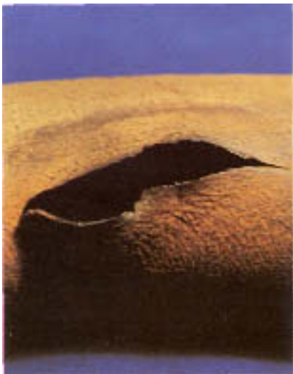
Figure 17.19 Rupture in an economizer tube caused by severe localized external-surface erosion associated with particulate matter entrained in flue gas.
