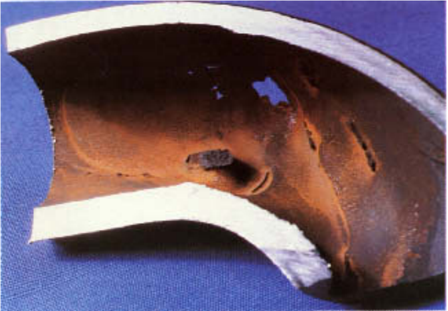
Figure 17.15 Elliptical metal-loss pattern and intact island of tube metal at perforated superheater U-bend. Erosion was caused by an object left in the tube 10 months earlier.
