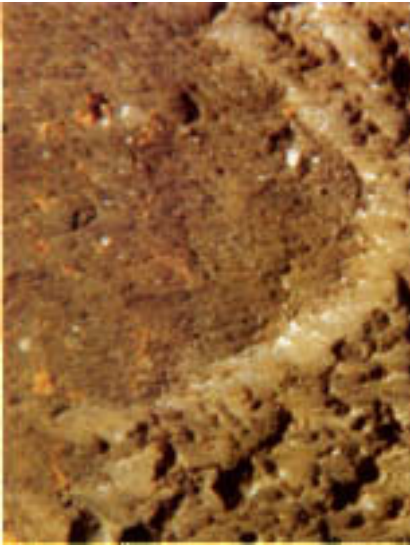
Figure 17.18 Erosion patterns at edge of wasted area. As in Fig. 17.17. Note flow patterns. (Magnification: 7.5X.)
