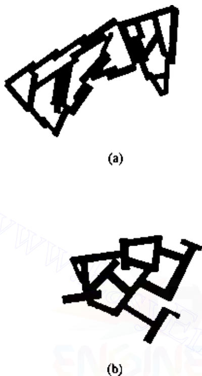
Figure 1.20 (a) Salt and (b) nonsalt flocculation of clay particles.
