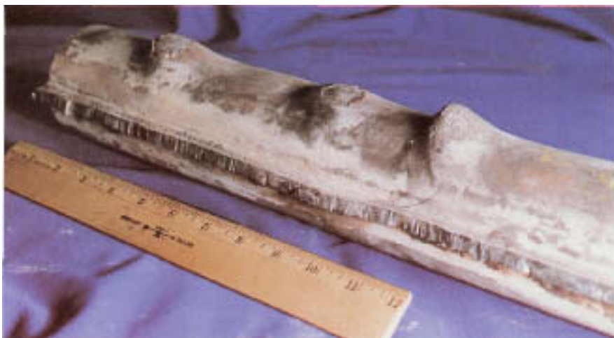
Figure 2.2 Multiple, abrupt bulges on the hot face of a waterwall tube of a recovery boiler.
