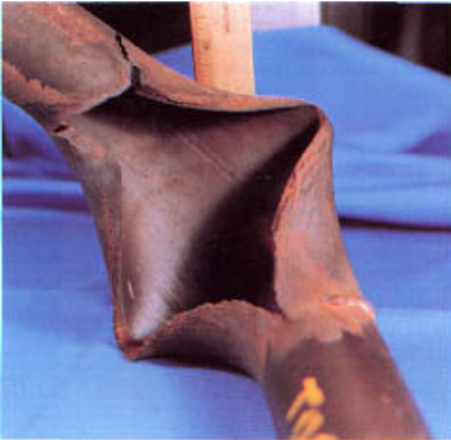
Figure 2.15 Massive thick-walled fracture caused by creep. Note the circumferential weld just below the failure. The tube is torn and bent to a 90° elbow by the violence of the rupture.
