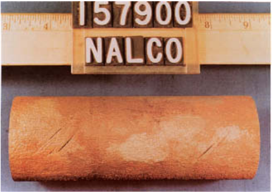
Figure 2.10 Spiral through-fissures due to chain graphitization. These fissures formed along lines of maximum shear stress.
