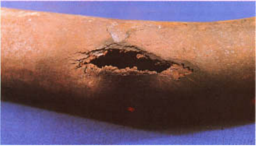
Figure 2.7 A small, ragged creep rupture at the apex of a bulge. Note the small secondary fissures and the relatively thick rupture edges.
