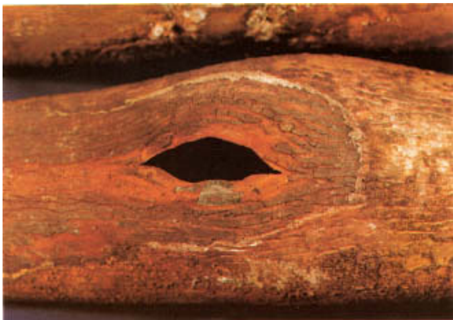
Figure 2.14 As in Fig. 2.13. Fragmented thermally formed oxide surrounds the rupture.
