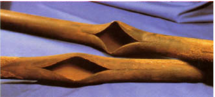
Figure 2.8 Two superheater tubes from a utility boiler [1400 psi (9.7 MPa)], failed by creep. Note the fish-mouth ruptures. Compare with Fig. 2.7.
