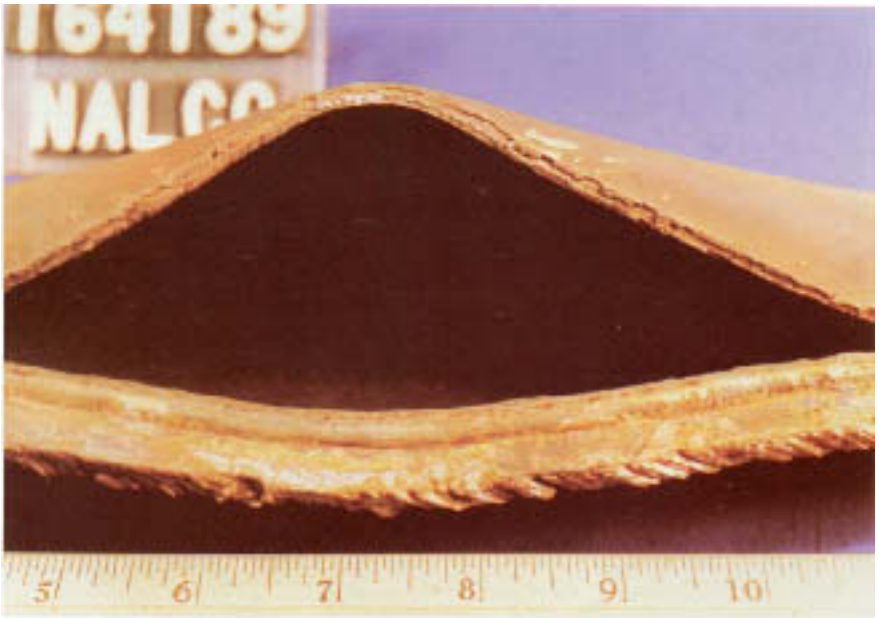
Figure 2.9 Rupture at longitudinal weld due to chain graphitization. Note the blunt, rough rupture edge. Such failures occur after long-term mild overheating.
