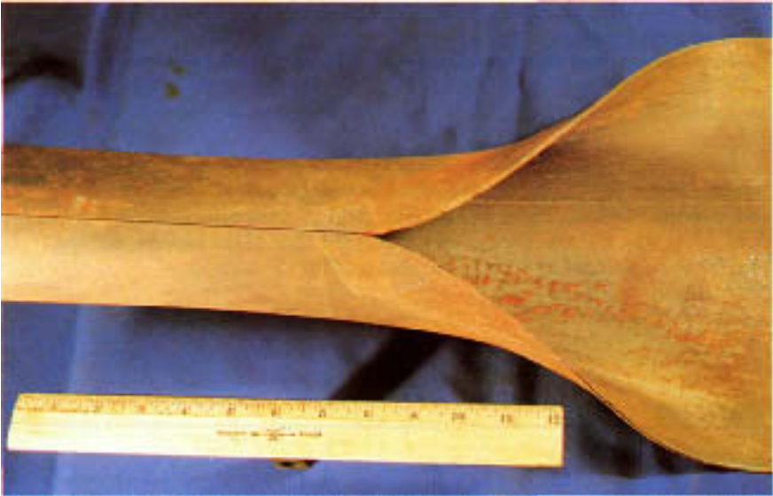
Figure 3.6 Longitudinal fissure running from the edge of a large, wide-open rupture.
