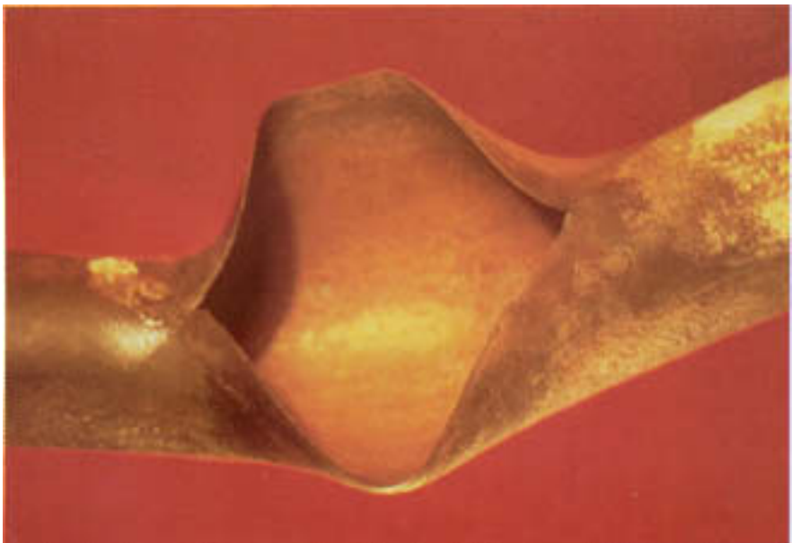
Figure 3.2 Short-term overheating in which bulging occurred before rupture. Note the chisel-like rupture edges.
