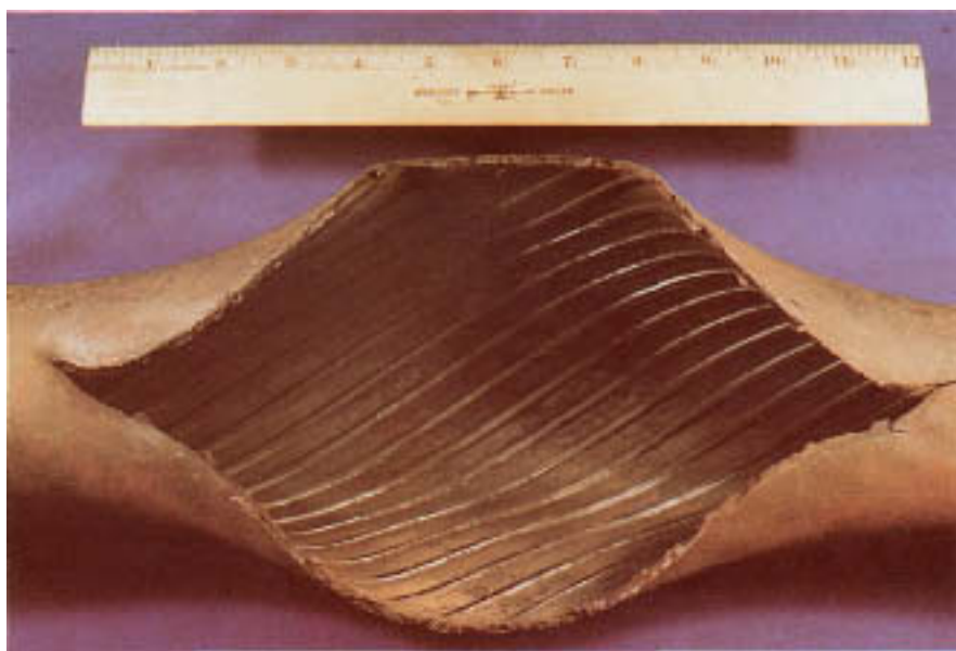
Figure 3.5 Large, fish-mouth rupture of rifled nose-arch tube. Rupture edges are thick, blunt, and ragged. Note the absence of significant deposits.
