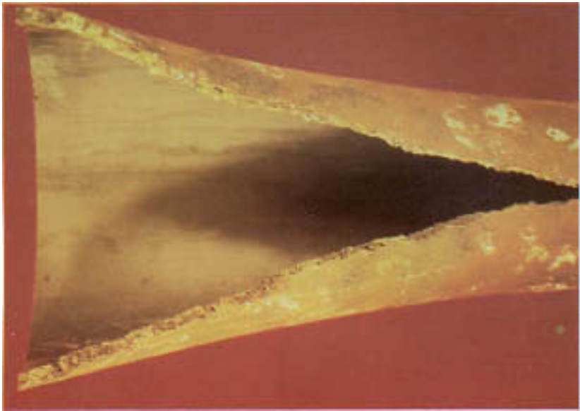
Figure 3.1 Longitudinal rupture in a superheater tube caused by partial pluggage upstream of failure, which in turn caused short-term overheating. Note the thick-walled rupture edges. Virtually identical tube circumferences are present at the rupture and away from the burst. Such failures often occur when temperatures exceed 1350°F (730°C).
