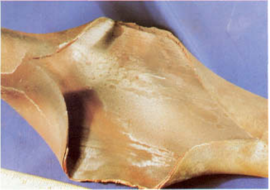
Figure 3.3 Violent rupture caused by short-term overheating. The tube is bent almost to a right angle, caused by the severity of the burst.
