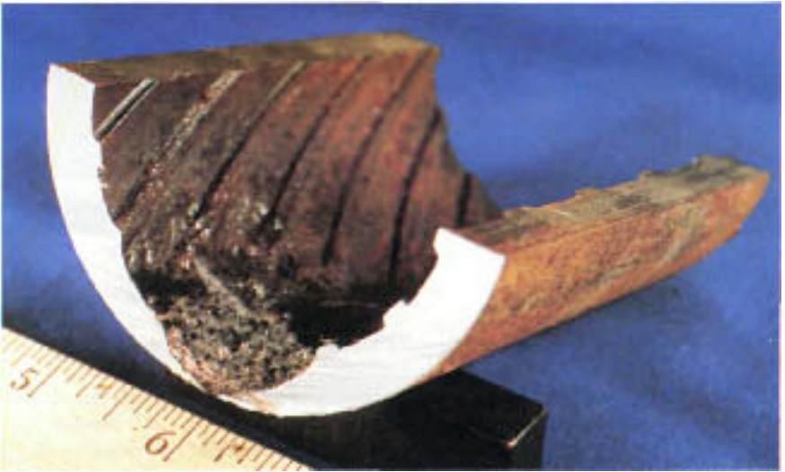
Figure 4.10 Perforation at bottom of crater.
