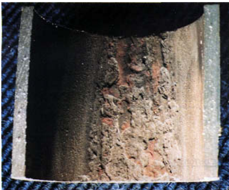
Figure 4.14 Internal surface showing wasted metal.
