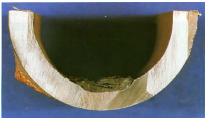
Figure 4.8 Cratered region beneath patch of iron oxides.
