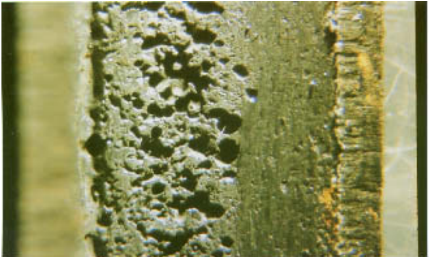
Figure 4.12 Band of hemispherical pits adjacent to groove. (Magnification: 6.5X.)
