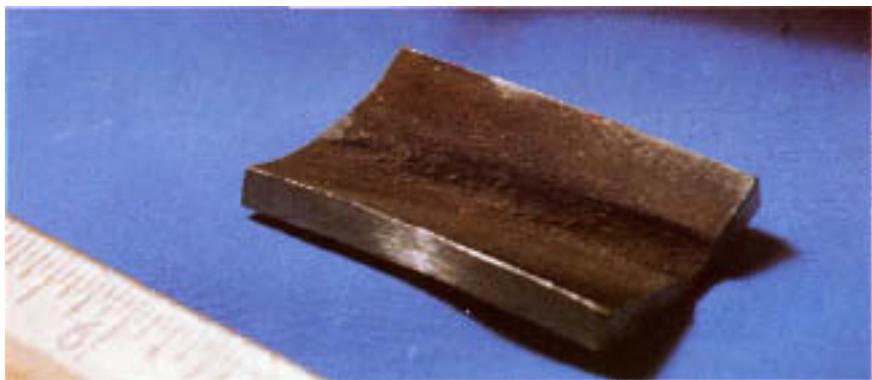
Figure 4.13 Grooved window section cut from inner bend.
