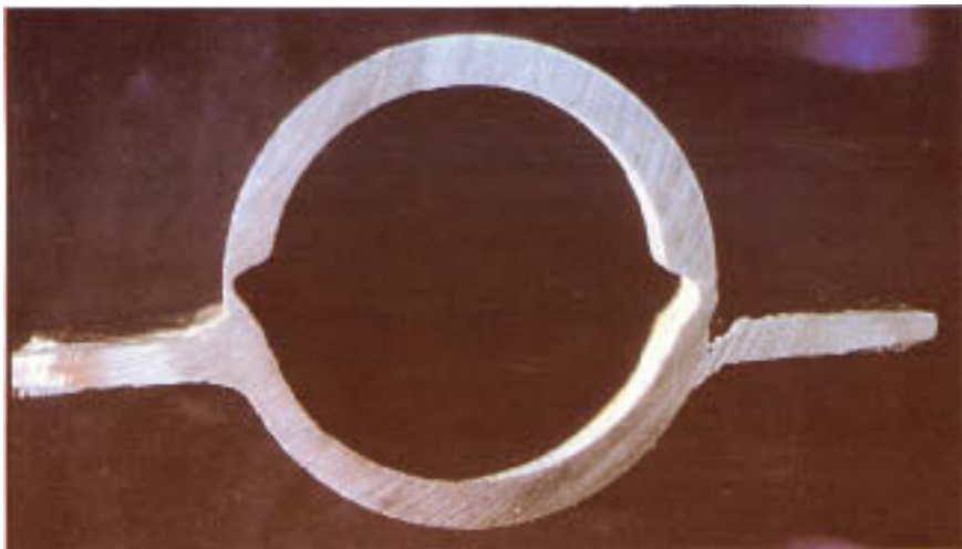
Figure 4.4 Caustic gouging along a longitudinal waterline. (Courtesy of National Association of Corrosion Engineers.)
