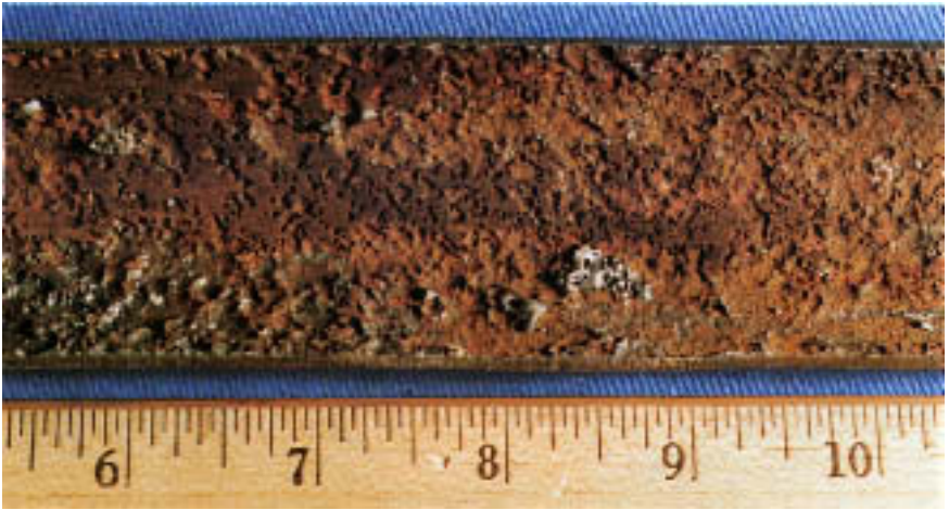
Figure 5.6 Internal surface of downcomer tube.
