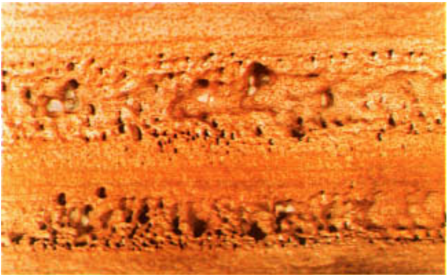
Figure 6.7 Contour of groove after deposit removal. (Courtesy of Electric Power Research Institute.)
