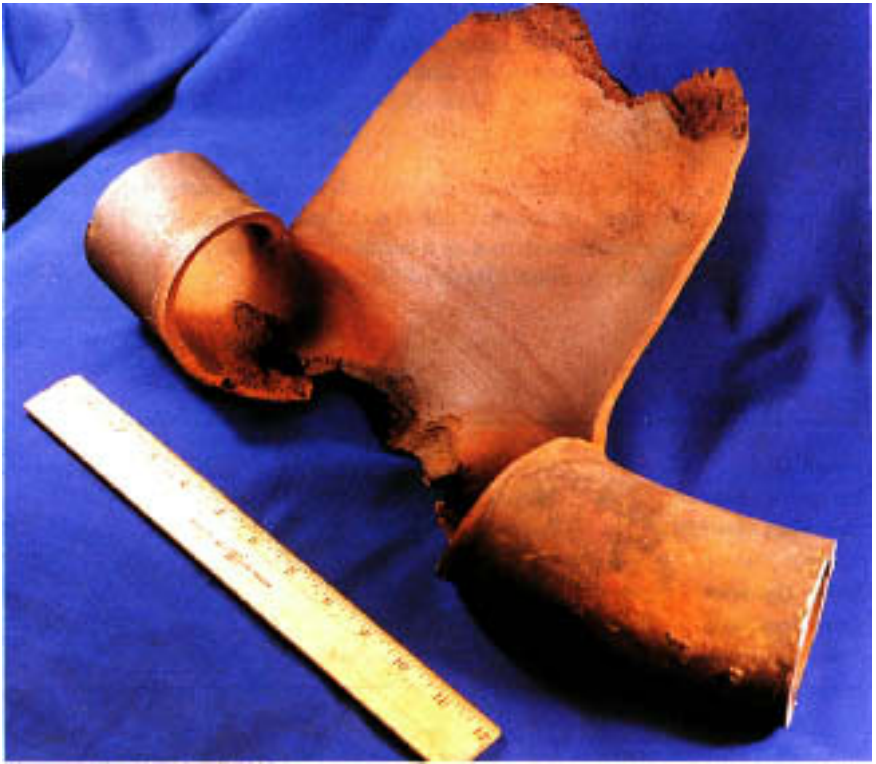
Figure 6.3 Rupture associated with low-pH gouging.
