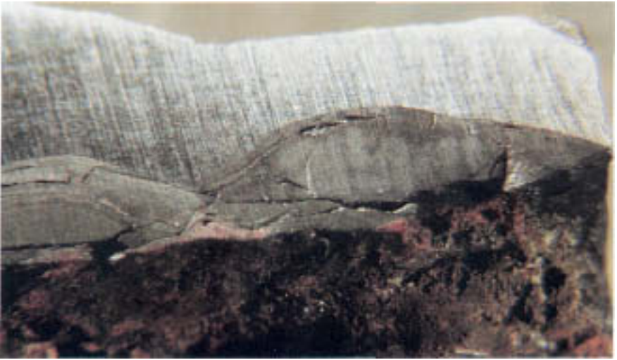
Figure 6.2 Deep gouge on internal surface. (Magnification: 7.5X.)
