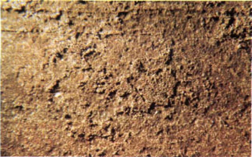
Figure 7.7 Appearance of attack by citric acid. (Magnification: 7.5X.)
