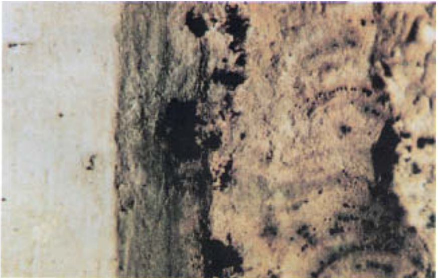
Figure 7.12 Acid attack along weld on internal surface. (Magnification: 7.5x.)
