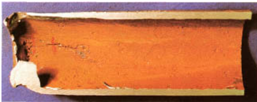
Figure 7.5 Longitudinal fissures near rolled end.
