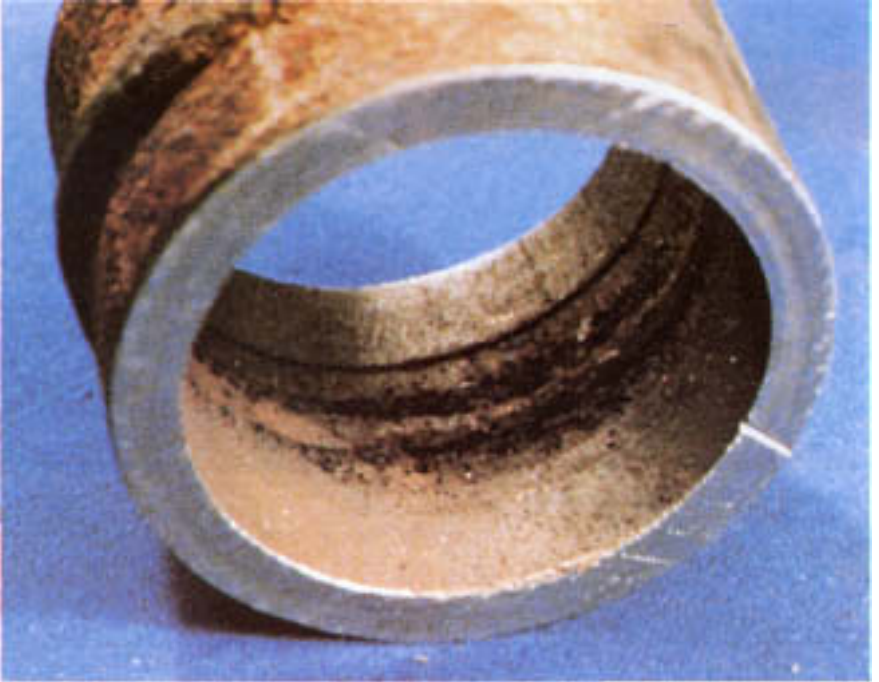
Figure 7.9 Acid corrosion at weld.
