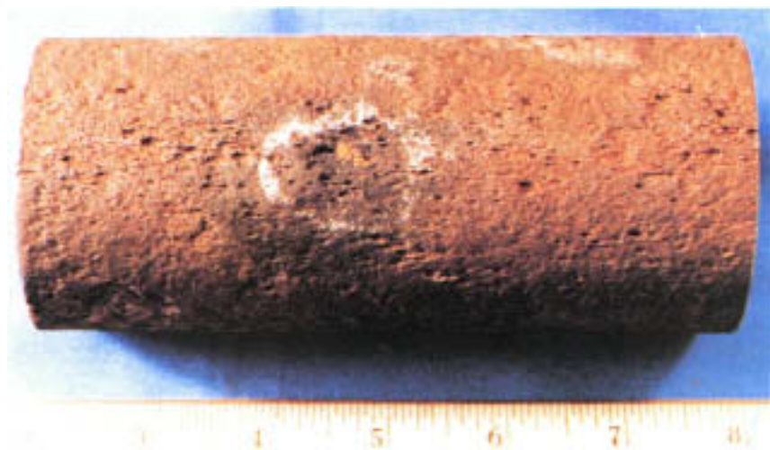
Figure 7.13 Acid corrosion on the external surface of a fire tube.
