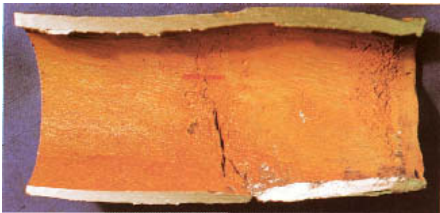
Figure 7.6 Transverse fissures near rolled end.
