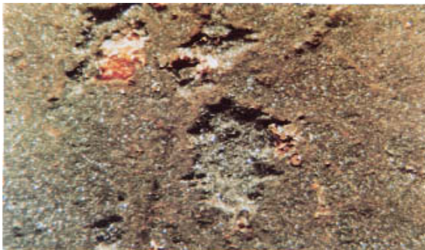
Figure 7.11 Metal loss from strong acid. (Magnification: 7.5X.)
