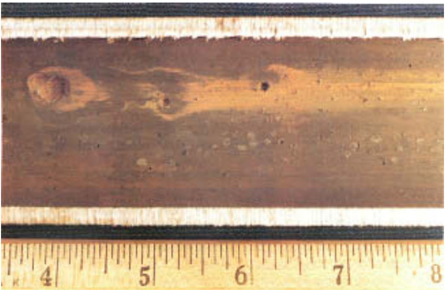
Figure 8.1 Oxygen pits in section of superheater tube. (Courtesy of Electric Power Research Institute.)
