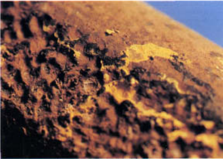
Figure 10.4 Contour of external surface in corroded zone. Note pockmarked surface appearance characteristic of attack on stainless steel.
