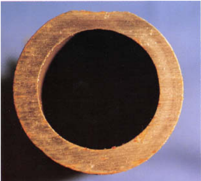
Figure 10.5 Transverse profile of tube showing metal loss.
