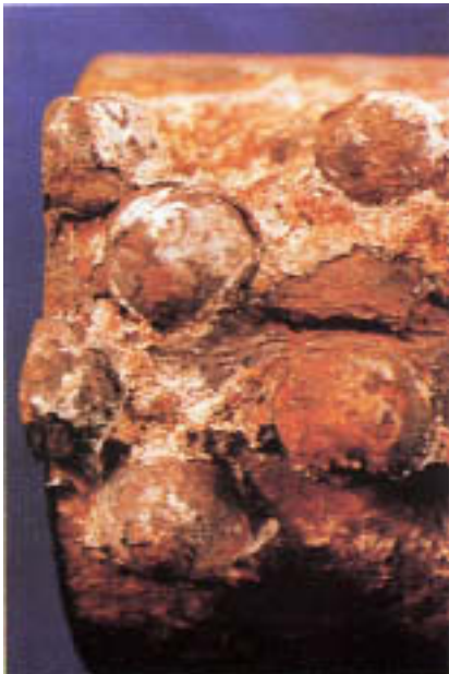
Figure 11.3 Longitudinal fissure adjacent to stud; fissure was caused by the combined effects of stresses imposed by internal pressure and the presence of a molten phase.
