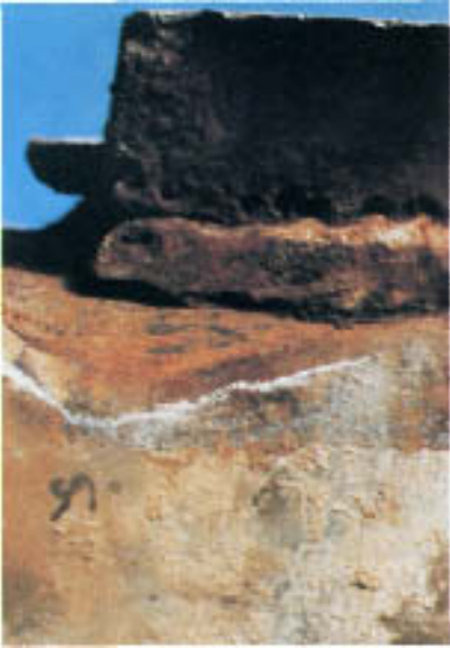
Figure 11.4 Metal loss around a fin resulting from exposure of a stainless steel-clad tube to a molten sodium salt.
