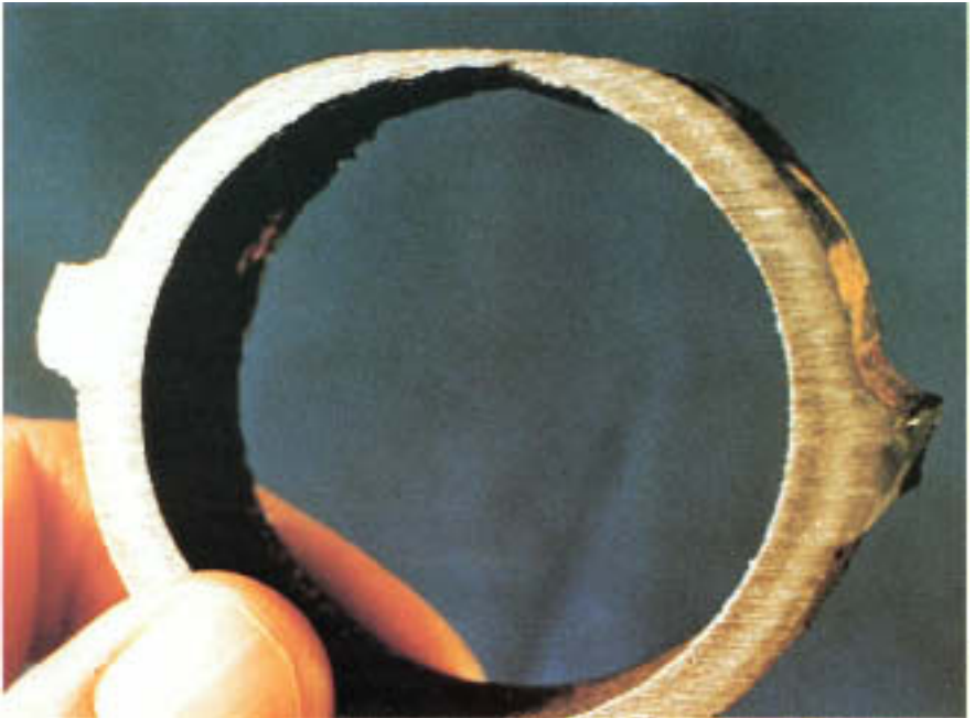
Figure 11.6 Severe metal loss along crown of tube resulting from exposure to a molten phase.
