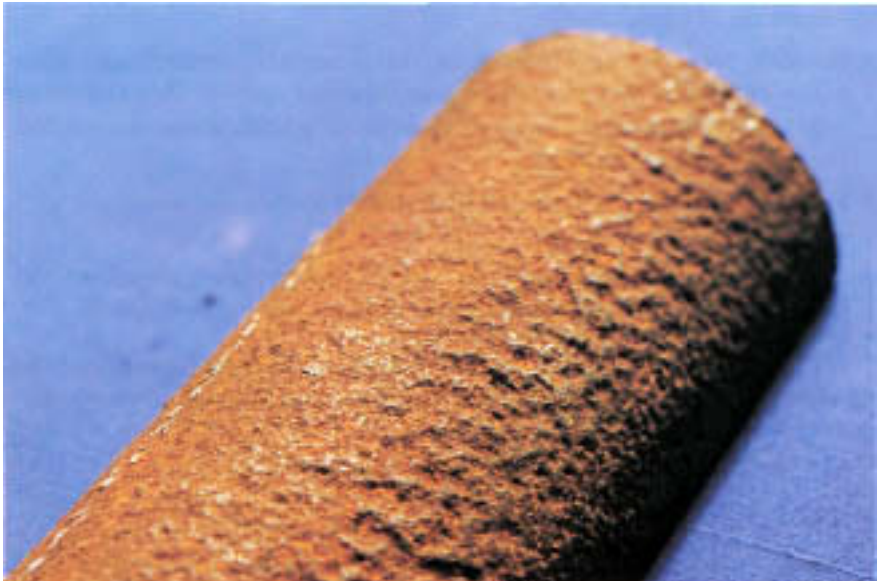
Figure 13.3 Appearance of the external surface of a screen tube after exposure to moisture and corrosive deposits during idle periods.
