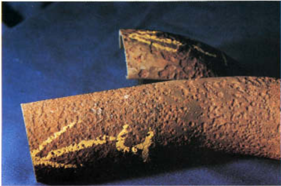
Figure 13.4 External surface of economizer tube following dew-point corrosion.
