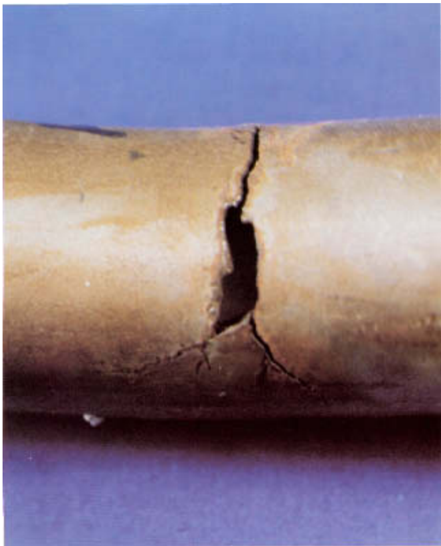
Figure 16.7 Transverse crack resulting from caustic stress corrosion in a bent stainless steel superheater tube. Note small “window” that has been blown out of the wall.
