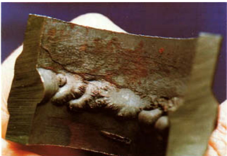
Figure 16.6 Appearance of crack on the internal surface. Note the branching and proximity to the weld bead.
