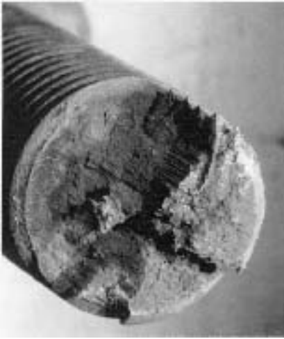
Figure 16.1 Steam drum bolt that failed by caustic stress-corrosion cracking. Note the typical brittle character of the fracture. ( Courtesy of National Association of Corrosion Engineers. )
