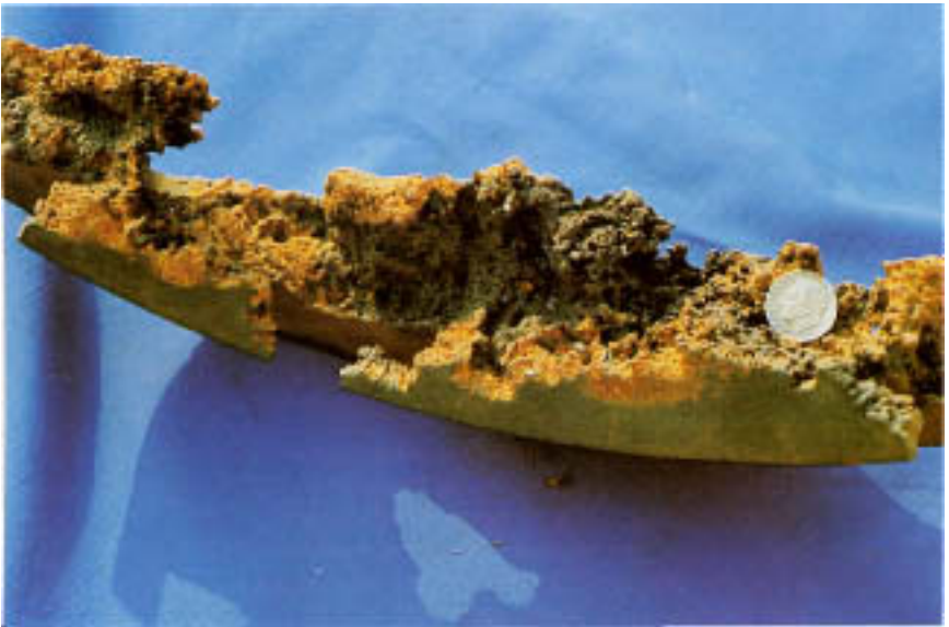
Figure 18.2 Pump-housing section severely attacked by cavitation. Material of the pump-housing section is gray cast iron.
