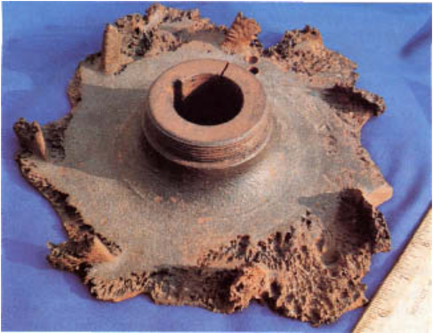
Figure 18.3 A cast steel feedwater-pump impeller severely damaged by cavitation. Note how damage is confined to the outer edges of the impeller where vane speed was maximum.
