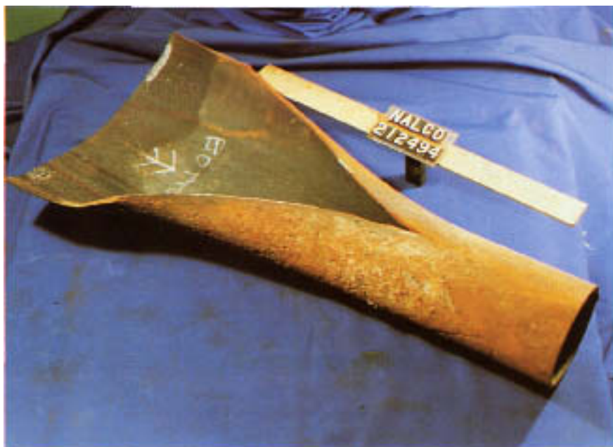
Figure 19.4 Massive rupture of tube along a weld-seam defect.
