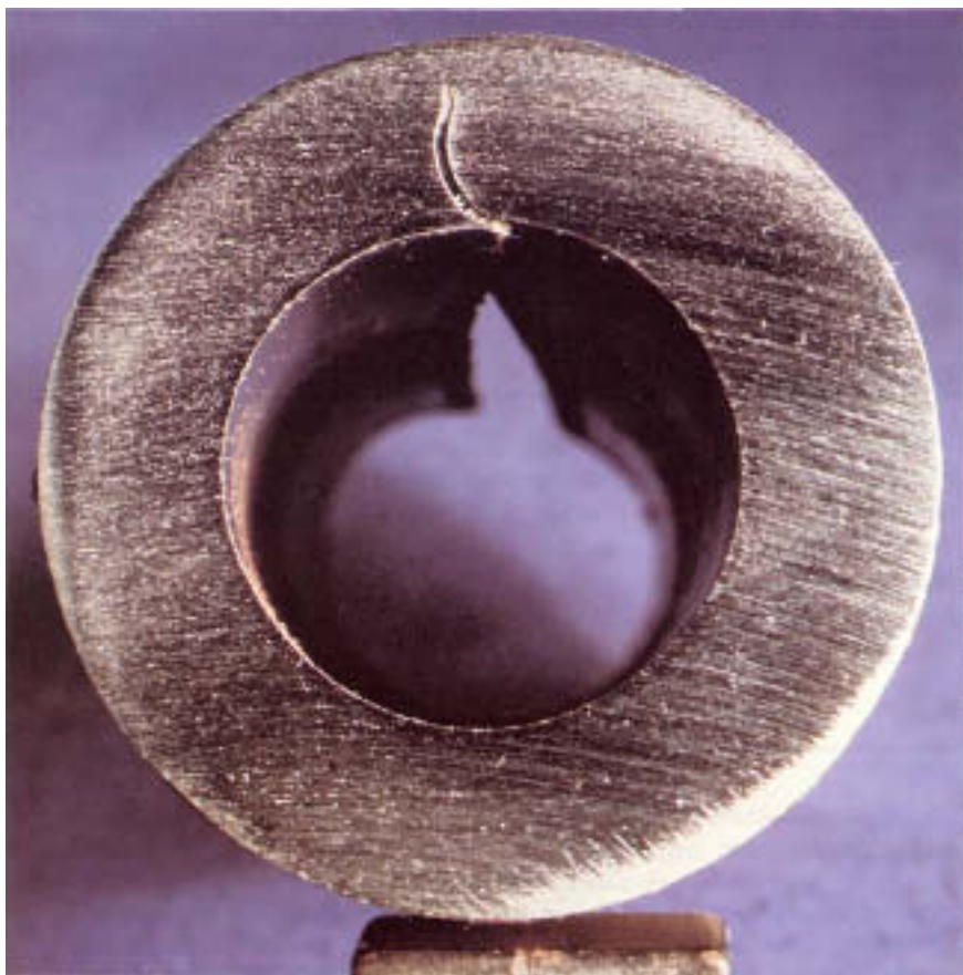
Figure 19.6 Failure along a massive manufacturing defect in the tube wall. (Courtesy of National Association of Corrosion Engineers.)
