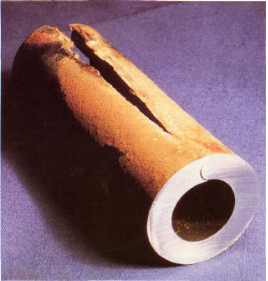
Figure 19.1 Curved defect originating on the internal surface of a seamless tube. This defect ran for 18 in. (45.7 cm) along the length of the tube. (Courtesy of National Association of Corrosion Engineers.)
