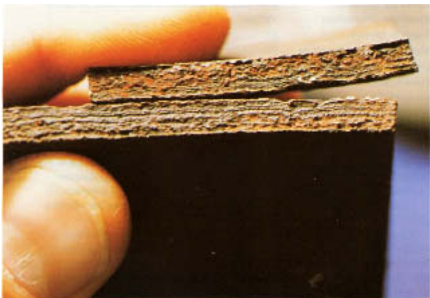
Figure 19.5 Edges of brittle rupture.
