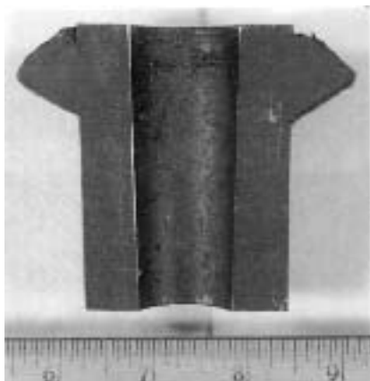
Figure 20.10 Fracture surface showing tube wall (inner ring) and fractured weld metal (outer ring).
