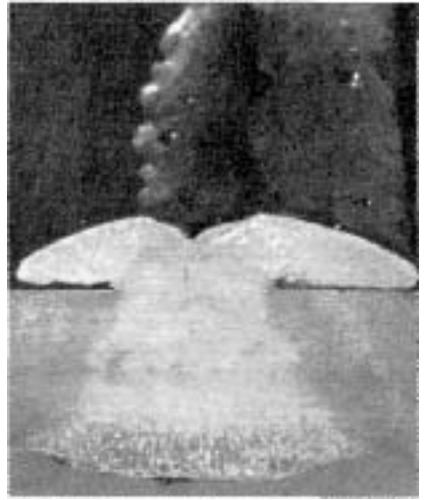
Figure 20.4 A burnthrough cavity formed on the backing ring of a tube weld. (Reprinted with permission from Helmut Thielsch, Defects and Failures in Pressure Vessels and Piping , New York, Van Nostrand Reinhold, 1965.)
