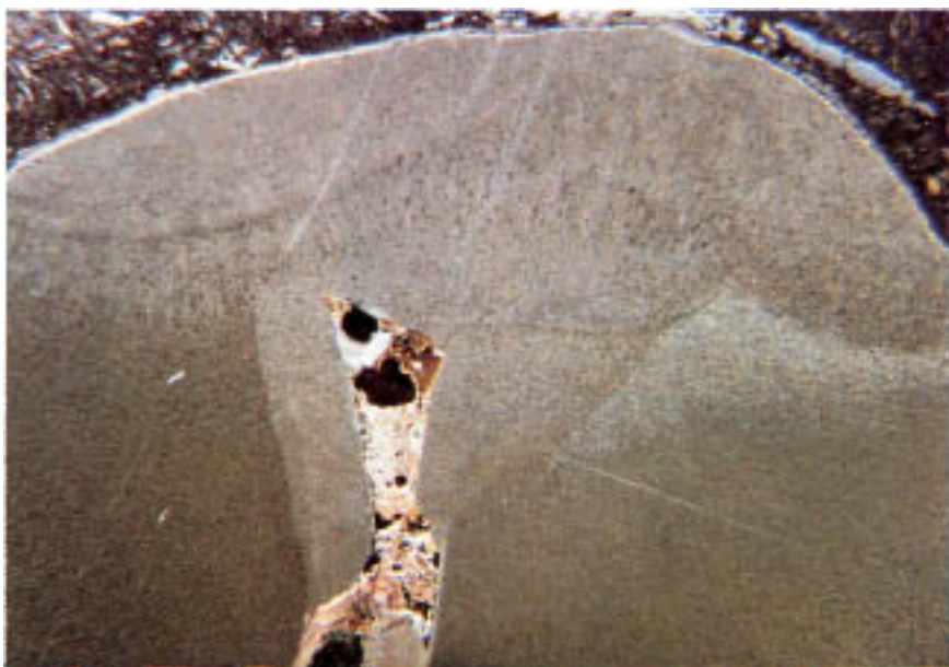
Figure 20.12 Cross section through window weld showing deep fissure in weld metal. (Magnification: 6X.)
