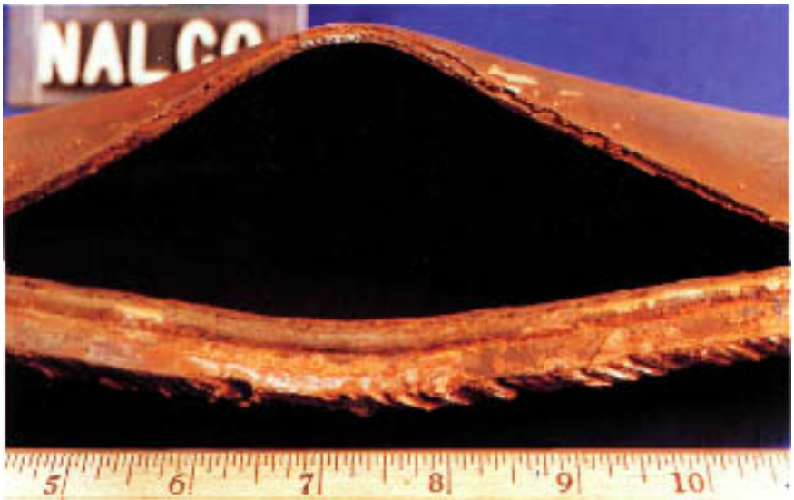
Figure 20.14 Massive fracture along weld bead resulting from weld-related graphitization. (Courtesy of National Association of Corrosion Engineers.)
