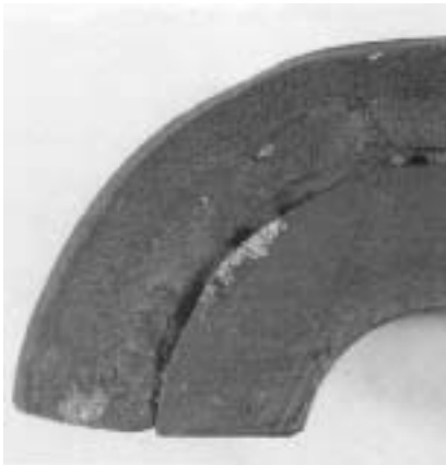
Figure 20.9 Cross section of tube showing weld metal (top of tube).
