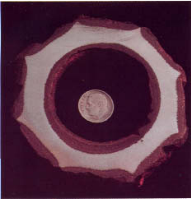
Figure 22.1 Pump impeller severely attacked by graphitic corrosion. Material of the impeller is gray cast iron. Note the gray areas on both internal and external surfaces where the metal has been converted to rust and graphite.
