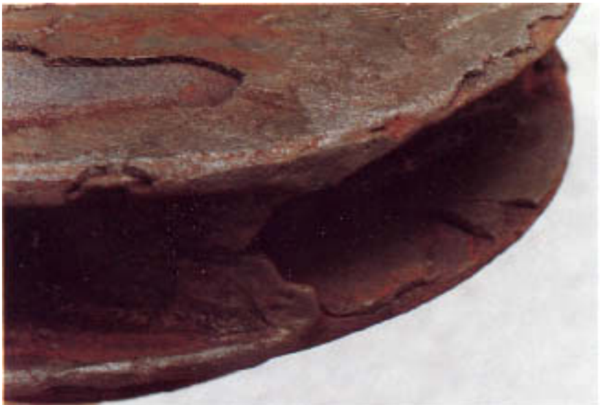
Figure 22.5 Severe graphitic corrosion of a gray cast iron feedwater-pump impeller. Patches of corrosion product have cracked and spalled, revealing uniform general wastage. Note the fracture in the impeller vane.
