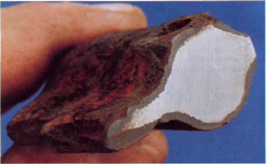
Figure 22.4 Graphitically corroded valve butterfly. Original surface contours are preserved. Edges, which were completely converted to brittle corrosion product, have broken.
