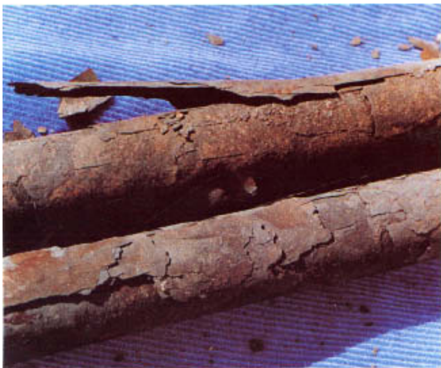
Figure 23.4 Peeling surfaces on a cupronickel high-pressure feedwater heater tube.
