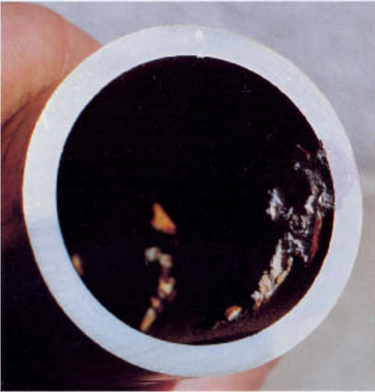
Figure 23.1 Plug-type dezincification beneath a deposit in admiralty brass tube.
