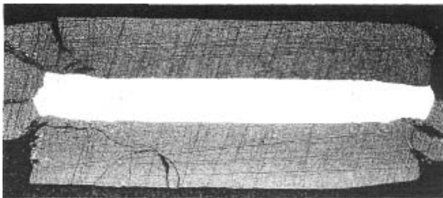
Figure 23.3 Cross section through a corroded Monel metal steam strainer. The dark area consists of oxides, sulfides, and elemental copper (Magnification: 15X.)
