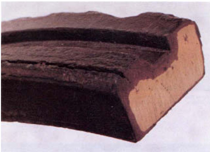
Figure 23.2 Layer-type dezincification of a brass pump component.
