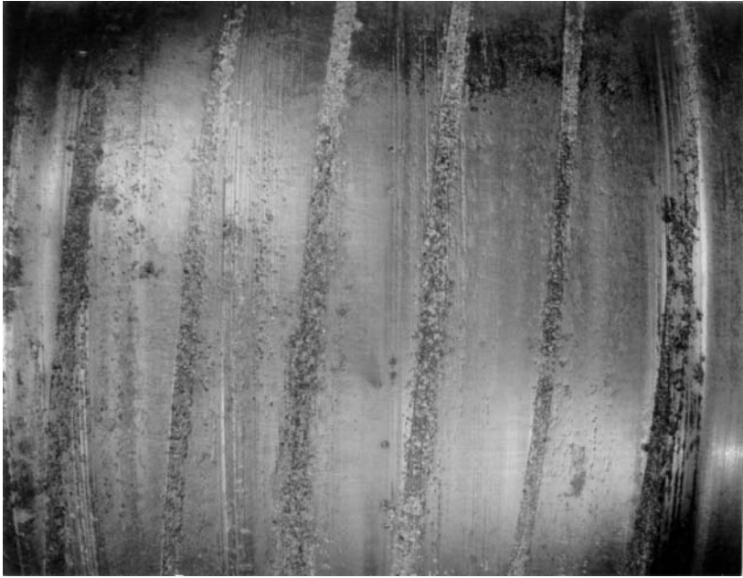
FIGURE 10 The three-body abrasive wear of a laser-hardened shaft sleeve in an abrasive service. Note the fine concentric scoring of the hardened surface. The helix pattern is the laser-beam overlapped zone produced by the laser process.
