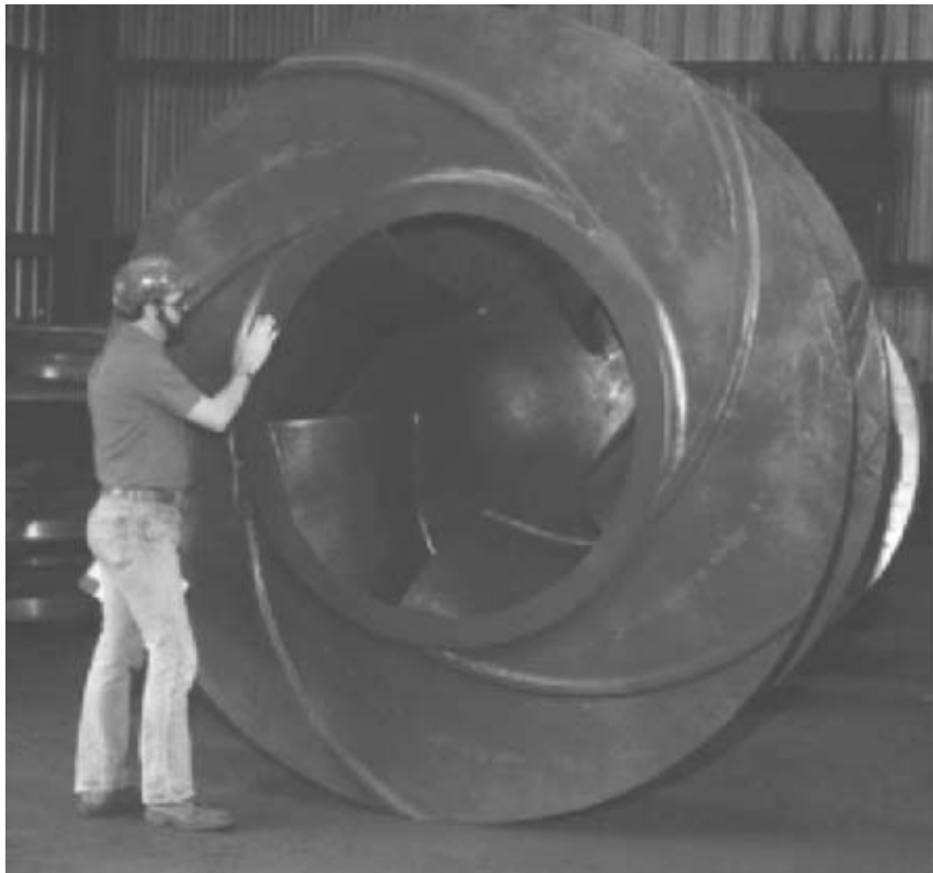
FIGURE 2 Dredge pump impeller, 105 in (2.67 m) diameter
