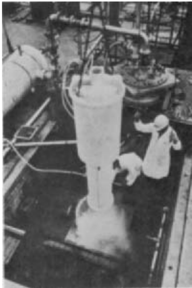
FIGURE 7 Multistage cryogenic pump on test stand (J.C. Carter Company, Inc.)
