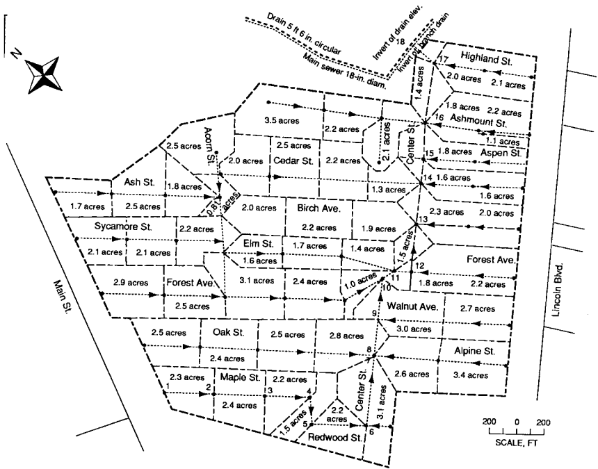
FIGURE C12.11 Map for storm sewer design example. (Adapted from Ref. 8.)
