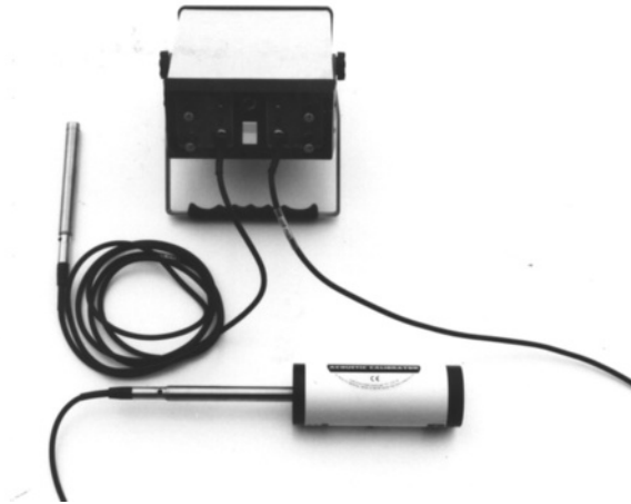
Figure 2.8 Laboratory grade condenser microphone equipment.
