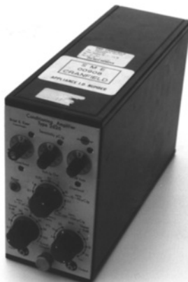
Figure 5.2 A typical charge amplifier — B&K Type 2626.
