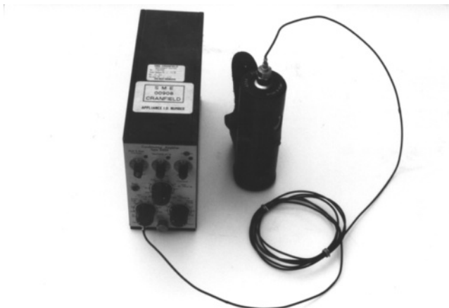
Figure 5.3 A field calibration exciter in action.
