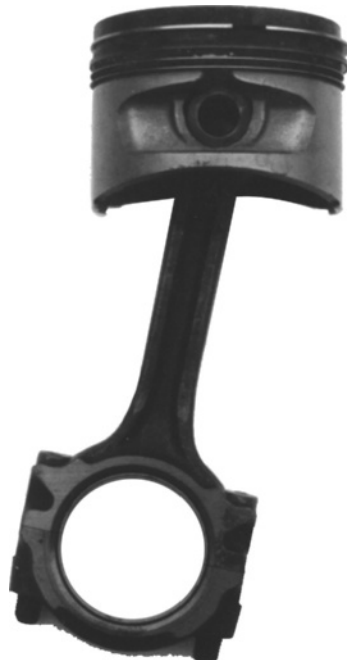
Figure 6.18 Photograph showing a typical piston and conrod assembly for a gasoline engine.
