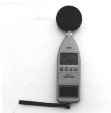
Figure 2.9 A typical sound level analyser.
