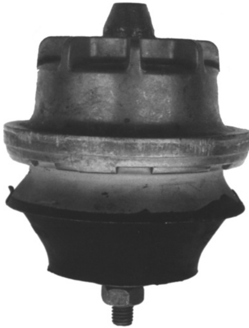
Figure 6.33 Photograph of a hydromount as fitted to a 4.0-litre V-6 gasoline engine in a full-sized luxury sedan.
