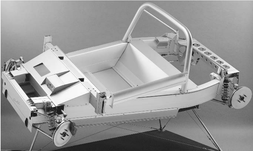
Figure 3.19 Punt chassis (courtesy of Lotus Cars Ltd).
