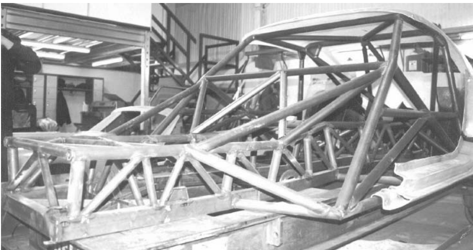
Figure 3.17 Triangulated sports car structure with integrated roll cage (Roots et al. 1995 with original permission from TVR Ltd).
