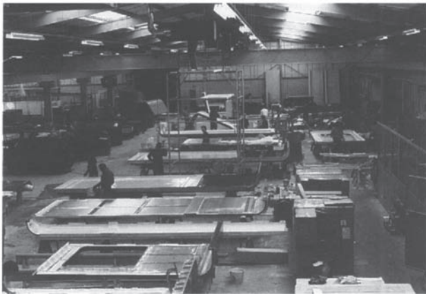
Fig. 2.6 Typical GRP production with large curing box at the rear of the factory.
