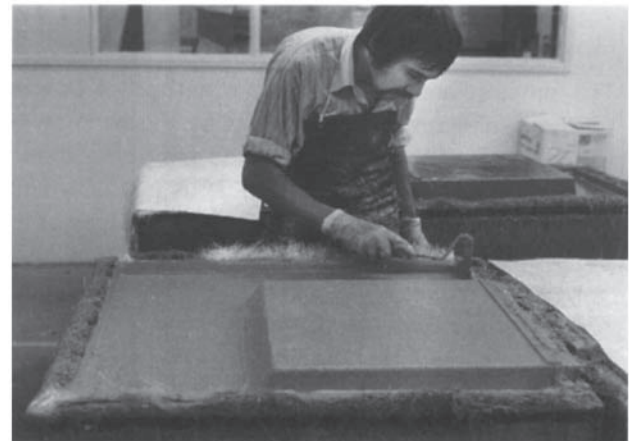
Fig. 2.4 Rolling out the lay-up to remove air bubbles.
