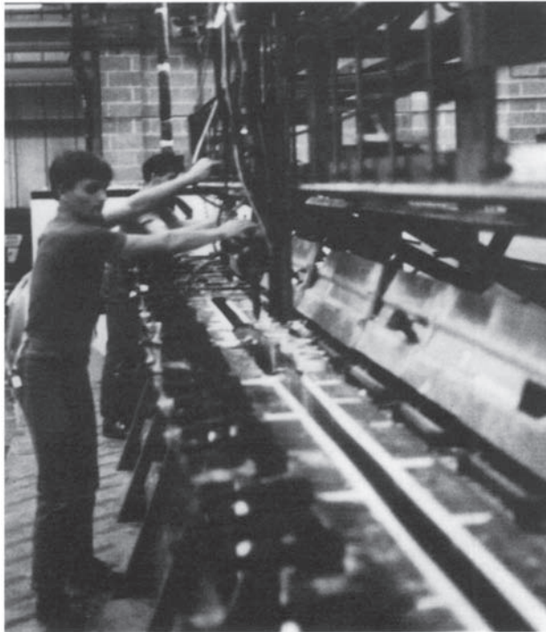
Fig. 5.18 Batch production of foamed panels—vertical foaming.
