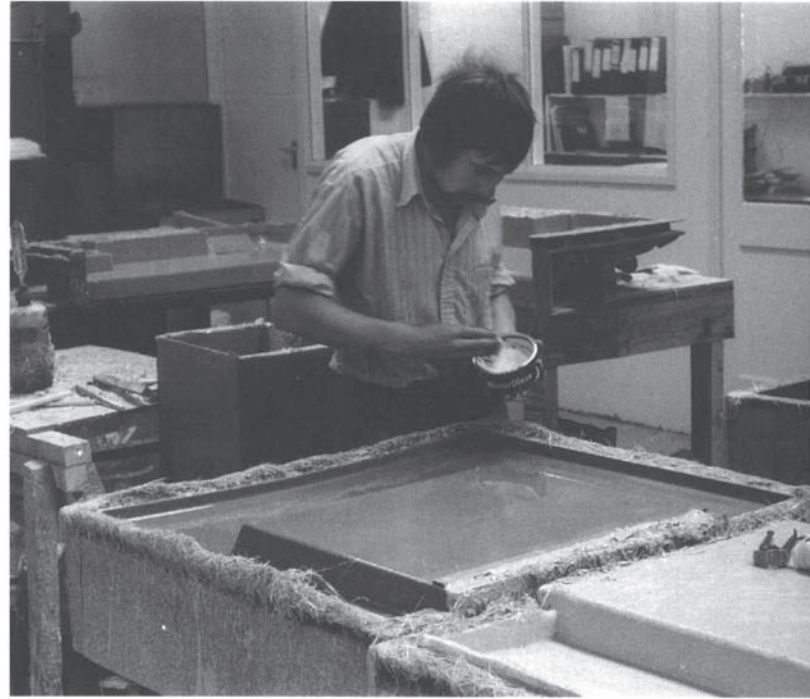
Fig. 2.3 Mould waxing prior to moulding.
