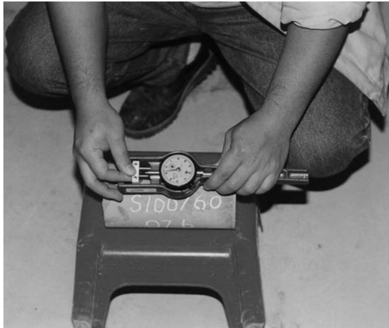
Figure 5-45 Free-drying shrinkage measurement using a Demac gage on a cylinder specimen
