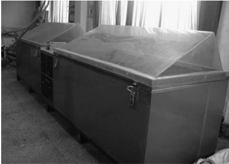
Figure 5-77 Seawater tank for marine environmental simulation test
