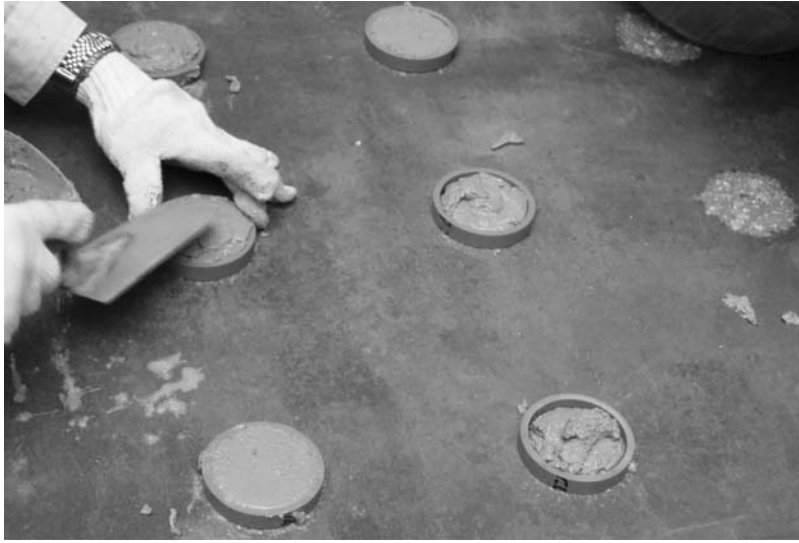
Figure 6-36 Casting of disk-like specimens for pull-off strength measurement
