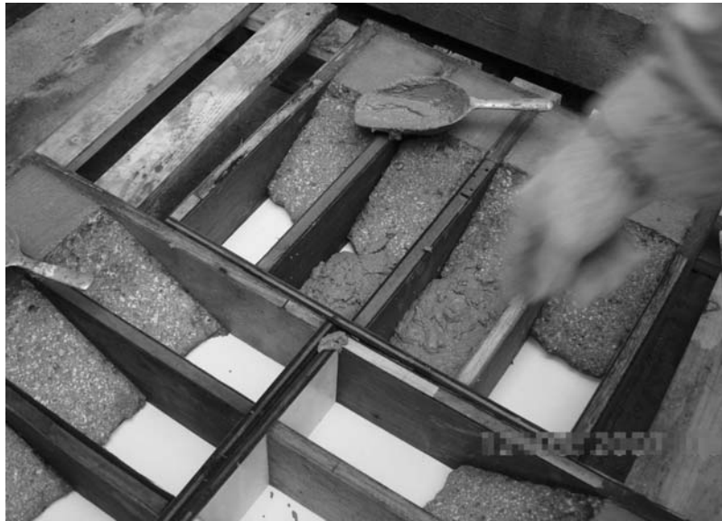
Figure 6-38 Casting of prisms for slant shear measurement
