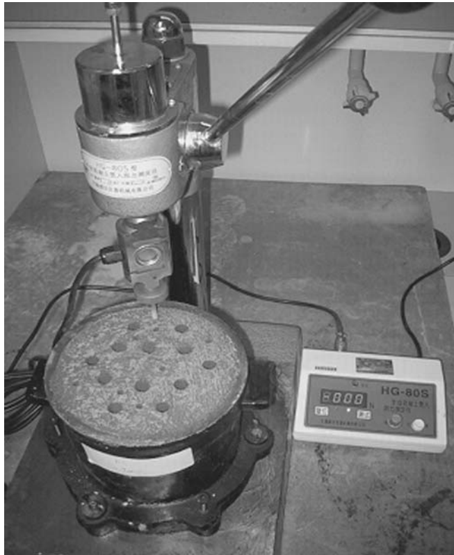
Figure 3-8 Measurement setup of concrete mixture setting time
