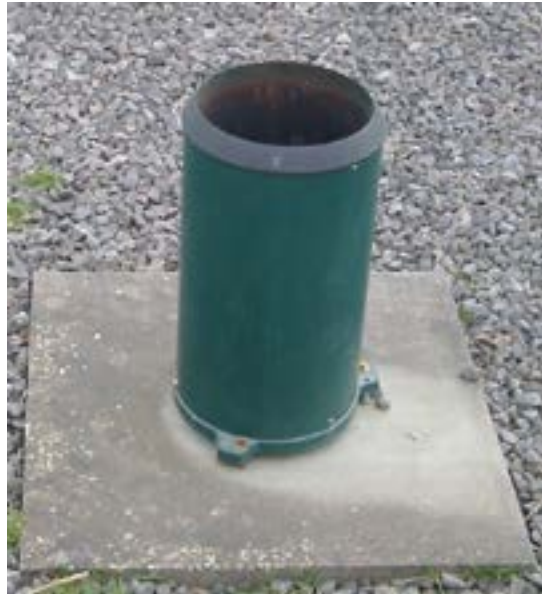
Figure 2 A typical rain gauge in the UK
